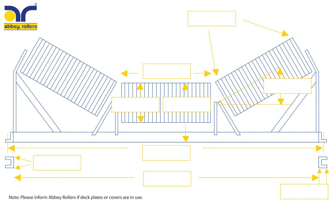
If the distance between the top of the centre roller and the underside of the base is less than 230mm , give the distance between stringer, as the base will have to be dropped to suit required height.
